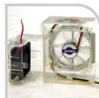
Optional fan guide provide better ventilation
