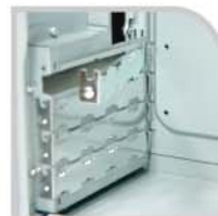
Screw-free PCI fingers
