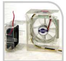
Optional fan guide provide better ventilation
