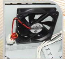
12 cm fan dissipates heat from CPU on top of case (Optional)
